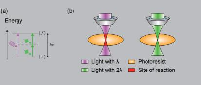
(a) Quantummechanical scheme of 1PP (magenta) and 2PP (green) (b) Reaction volumes in 1PP vs. 2PP: Only 2PP enables the confinement of the photoreaction to the tiny focal volume.
