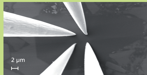
Measurement of electrical conductivity with special micromanipulators
