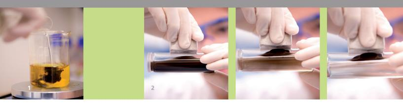
1 Fabrication of magnetic nanoparticles approx. 10 nm diameter 2 Separation of superparamagnetic microparticles from water
