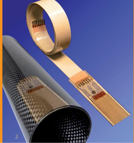
The fact that the transducers can alternately function both as receivers and as ultrasonic transmitters makes it possible to generate wavefronts at different points of the part and to check even the most inaccessible corners.
