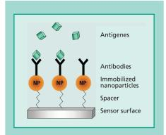
Multifunctional SiO<sub>2</sub>-based nanoparticles enable the conjugation of marker-specific antibodies or relevant antigens and are tailored to both the sensor system and the microfluidics of the diagnostic system.
