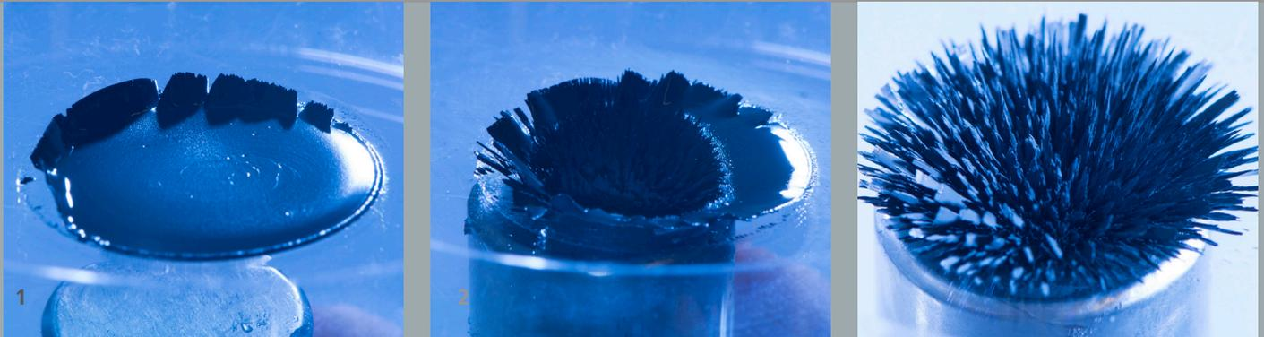
1 - 3 In a magnetic field, the MRF develops a fibrous structure, with tangled chains of particles along the field lines
