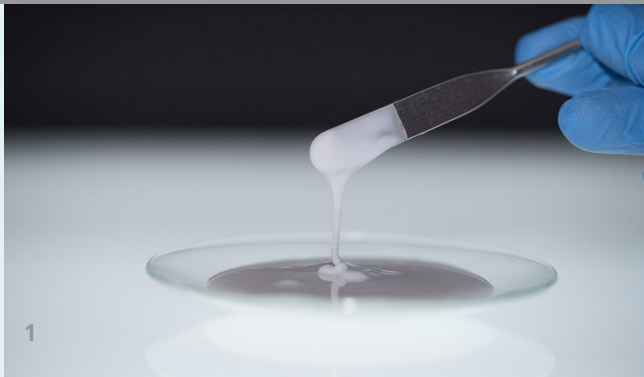
1 Glass paste for screen printing
