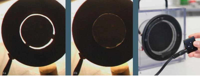
vantage of silicone is that its hardness can be varied widely by use of adjustable chemical cross-linking. By increasing the permittivity of the silicone, the expansion and actuation stress can be boosted.
