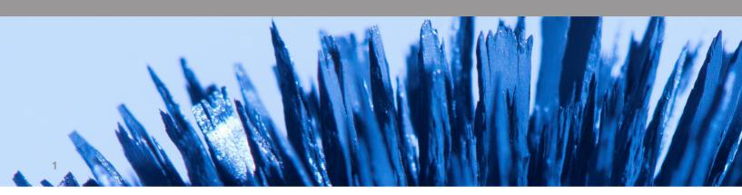
1 Activated Magnetorheological Fluid (MRF) with iron-particles alligned to magnetic field lines
