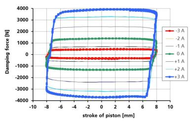
Damping force of the MRF damper with permanent magnet and electromagnet at various coil currents
