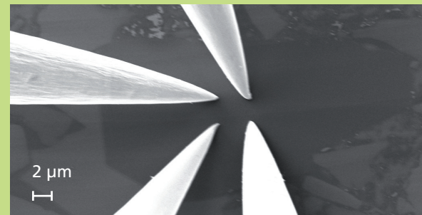
Measurement of electrical conductivity with special micromanipulators
