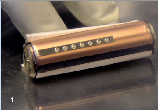
1-3 Opening a cell in an inert gas atmosphere and CT image of a standard lithium-ion battery
